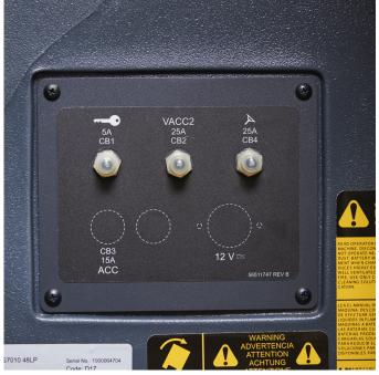
**4** Inspect the circuit breakers
