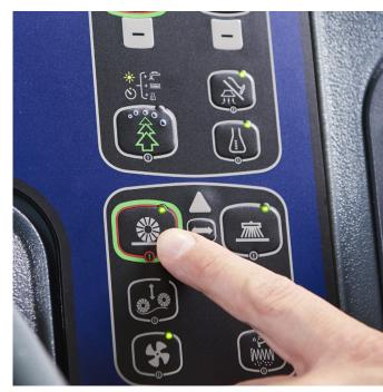
4 Adjust main broom pattern per operators manual to avoid overload condition. Inspect broom and drive for debris or adjust height if overload detected
