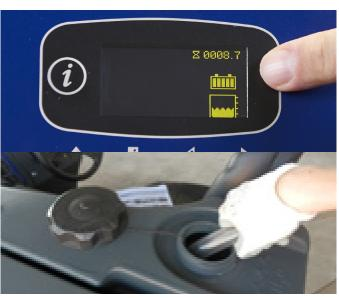
fill the tank with clean water. The clean water temperature must not exceed 40 °C
