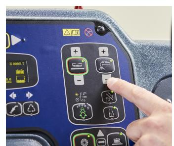
9. Adjust to the desired water flow
