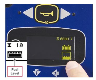
1. Check the Diesel fuel tank level / LPG bottle charge/Battery charge. In case re-fill/change the LPG Bottle / charge the batteries
