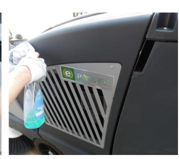
20. Clean the machine using a damp cloth and park it with the recovery tank open
